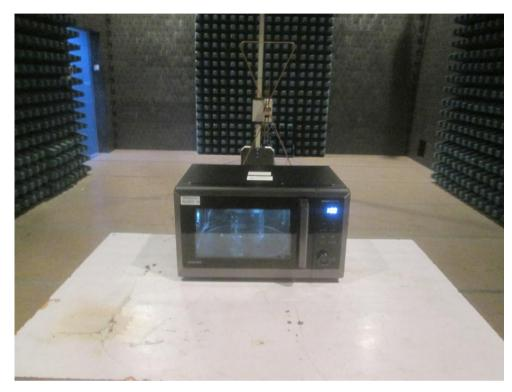
2. Radiated Emission Measurement above 1GHz
