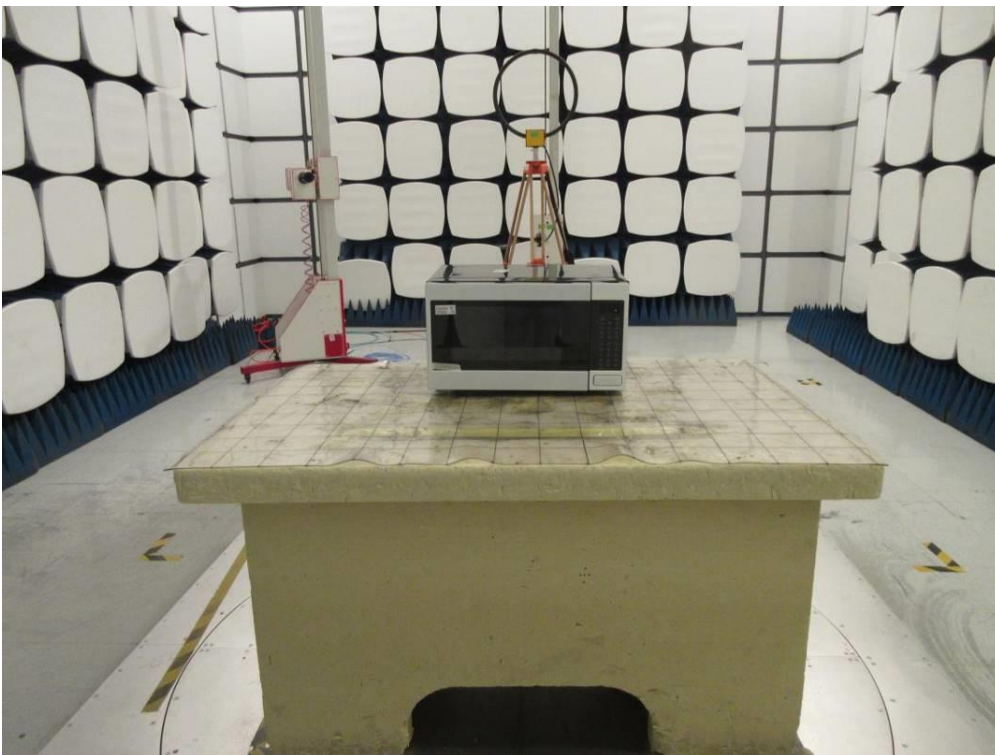
Radiated Disturbance above 9KHz-30MHz
