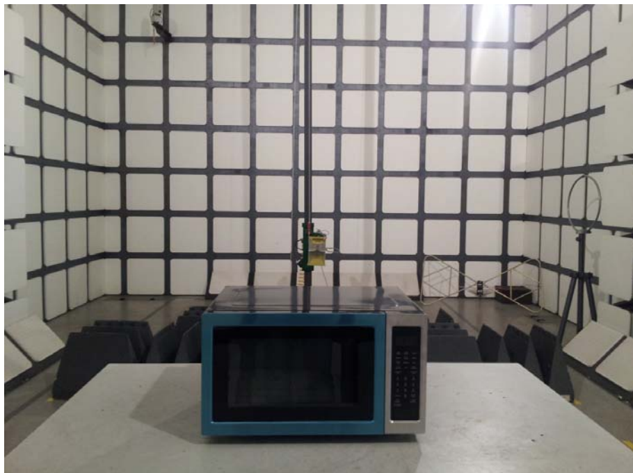
Operating Frequency Test Set-up:
