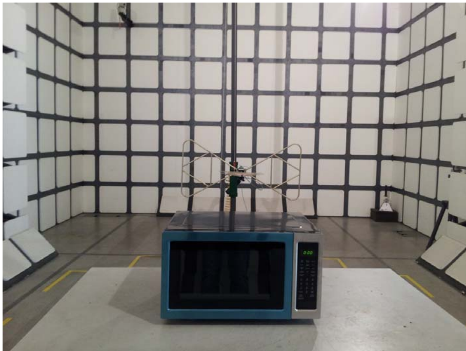
Radiated Emission Test Set-up (30~1000MHz):
