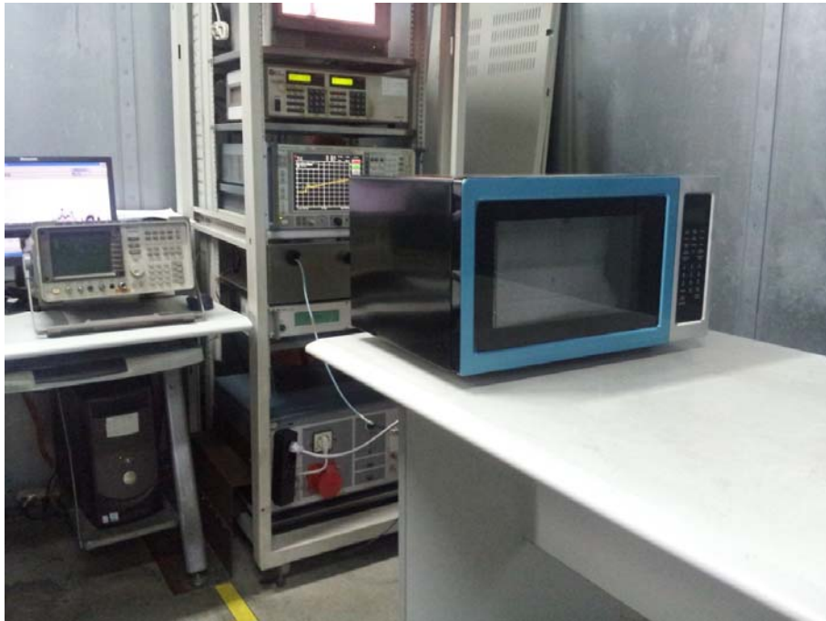
Conducted Emission Test Set-up:
