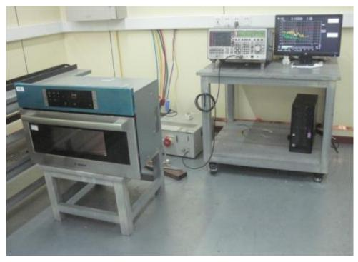
Radiated Emission Test Set-up (30 -1,000MHz):
