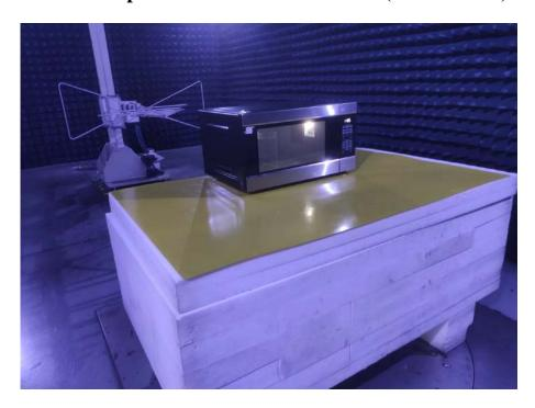
**Radiated Spurious Emissions Test View (Above 1GHz)**
