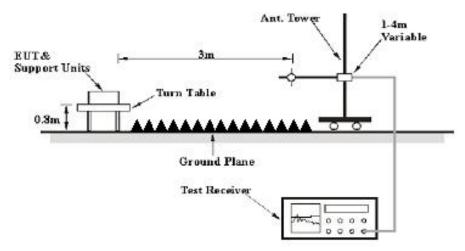
The radiated emission were performed in the 3 meters chamber test site, using the setup accordance with the FCC MP-5. The specification used was the FCC part 18 limits.
