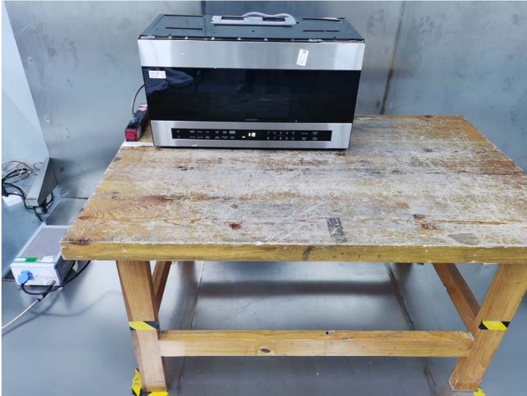
Conducted Emissions Side View
