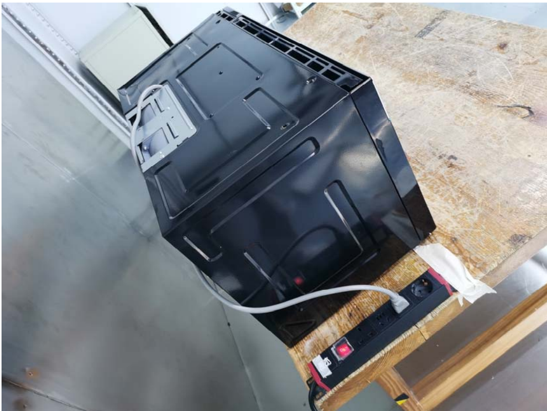
Conducted Emissions Side View
