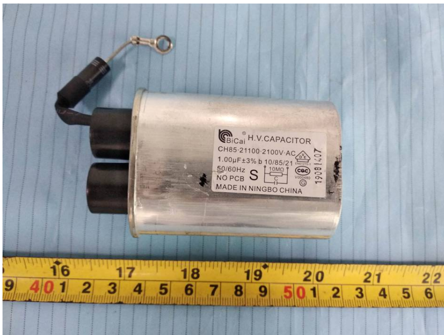
EUT – H.V. Capacitor Top View
