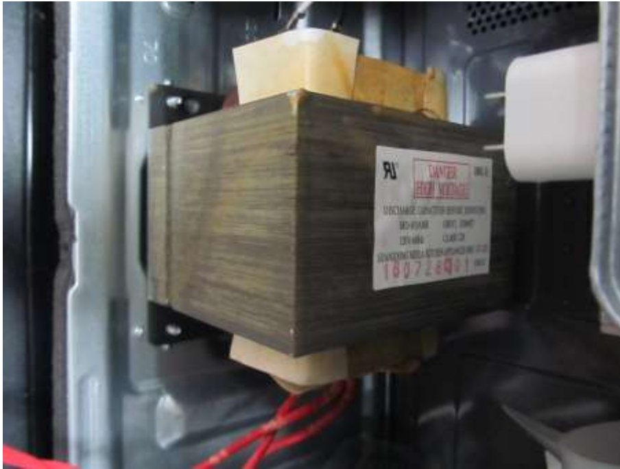
High-voltage Transformer View
