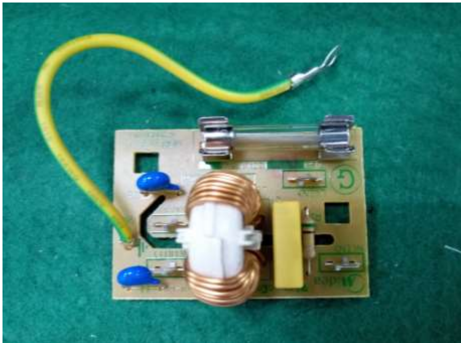
Power Filter Board -Top View
