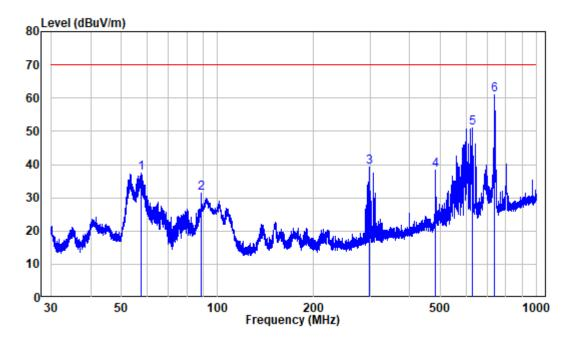
Site : chamber Condition: 3m VERTICAL Job No. : RA230625-36101E-EMA1 Test Mode: Microwave
