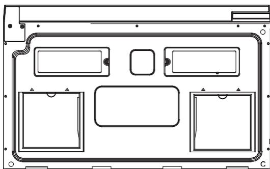
1. To remove the grease filter, pull the lever, then pull filter downward. The filter will drop out.
