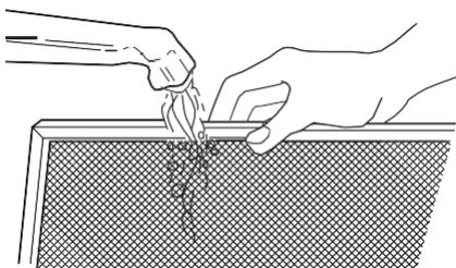
2. Soak the grease filter in hot water using a mild detergent. Rinse well and shake to dry or wash grease filter in dishwasher. It is best to place in upper rack of dishwasher for cleaning.
