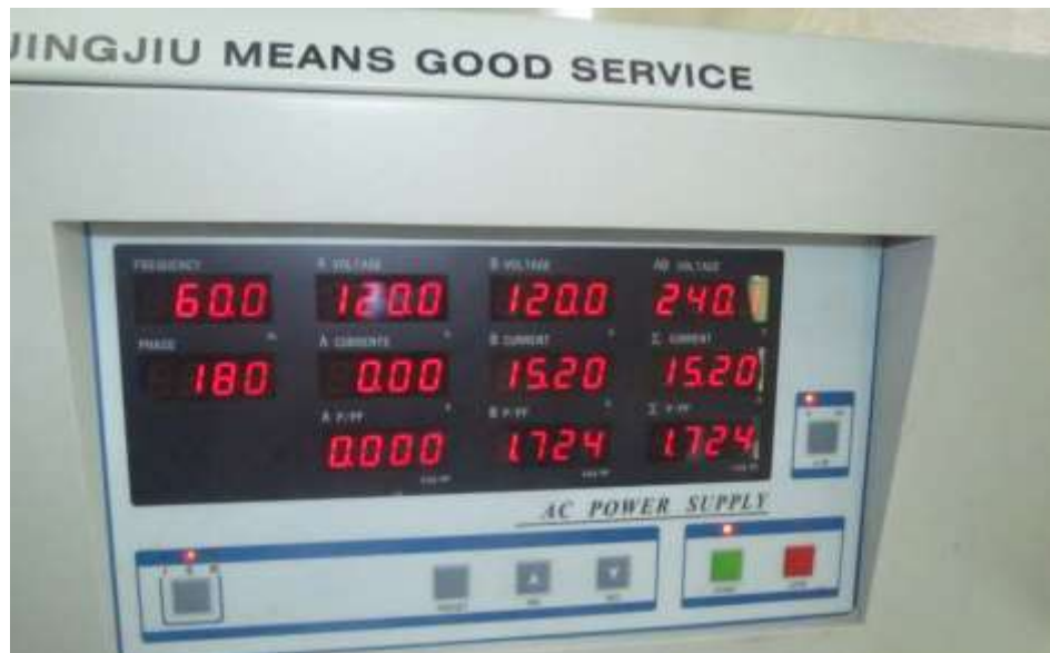
Input power Test Set up-240V
