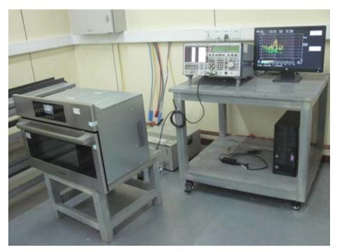
Radiated Emission Test Set-up (30 -1,000MHz):
