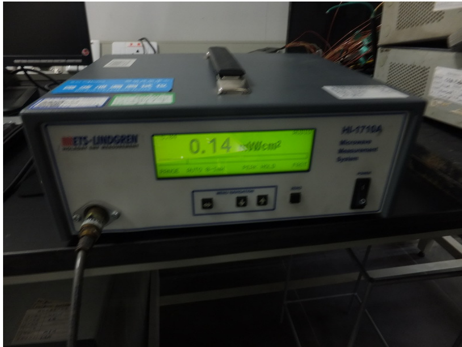
Radiation Hazard Test Set-up -240V
