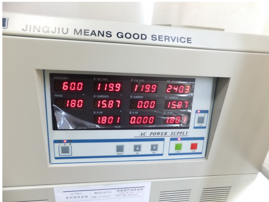
Input Power Test Set-Up (240V/60Hz)
