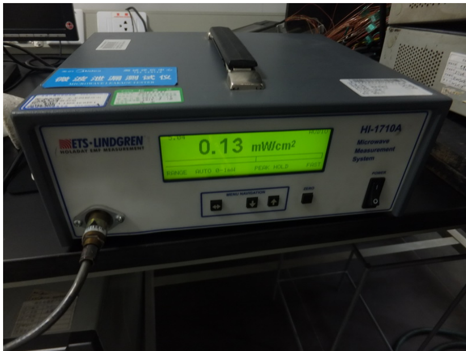
Radiation Hazard Test Set-up (208V/60Hz)
