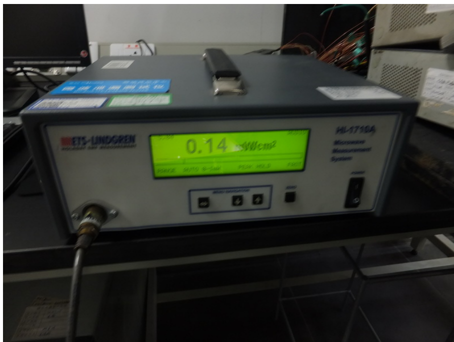
Radiation Hazard Test Set-up (240V/60Hz)
