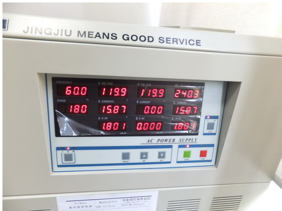
Input Power Test Set-Up (240V/60Hz)
