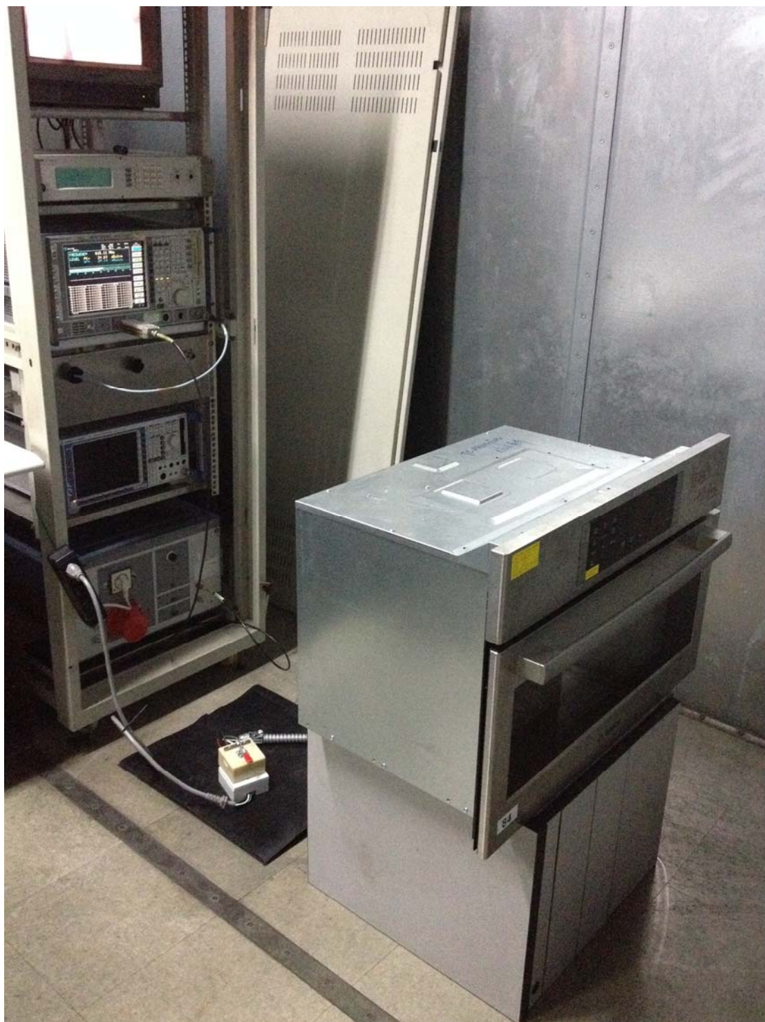
Conducted Emission Test Set-up
