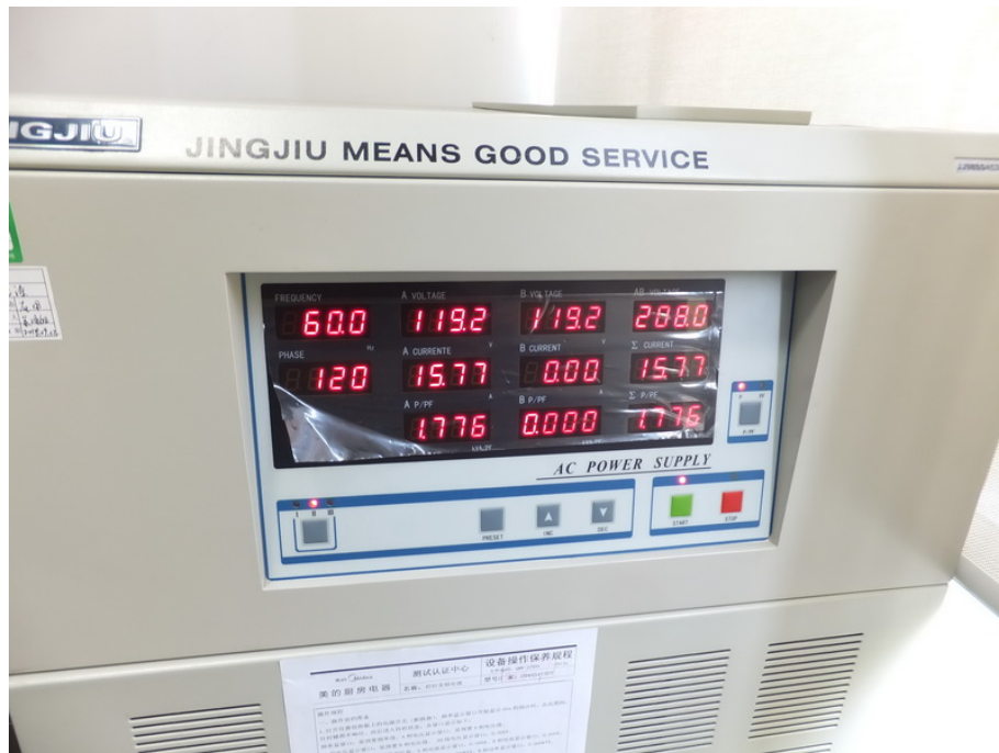
Input Power Test Set-Up (208V/60Hz)
