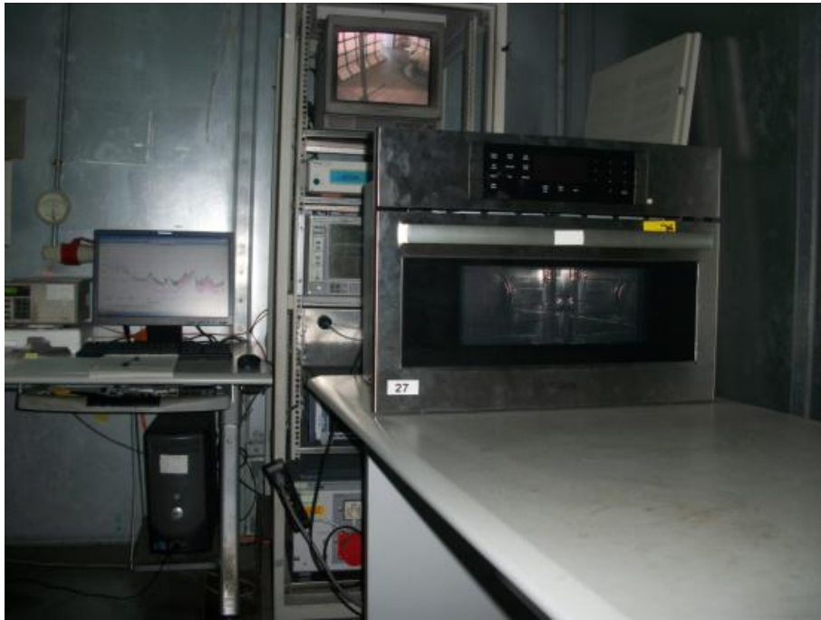
Conducted Emission Test Set-up
