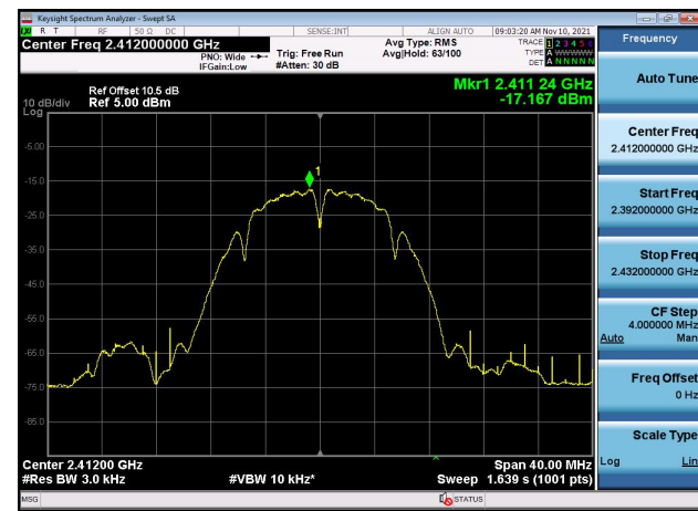
Power spectral density-802.11b ,2462MHz,Ant0
