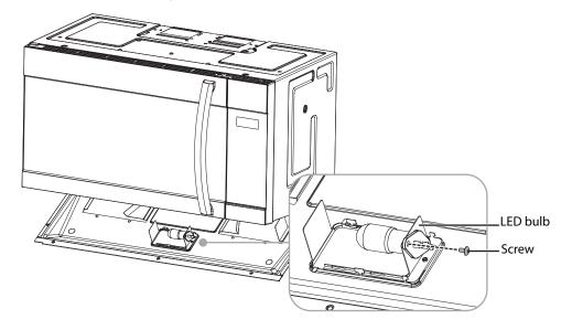
4 Replace the base plate and secure it with the screws.
