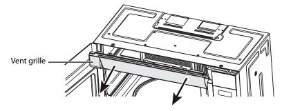
4 Replace the charcoal filter. Make sure that the wire mesh is visible from the front.
