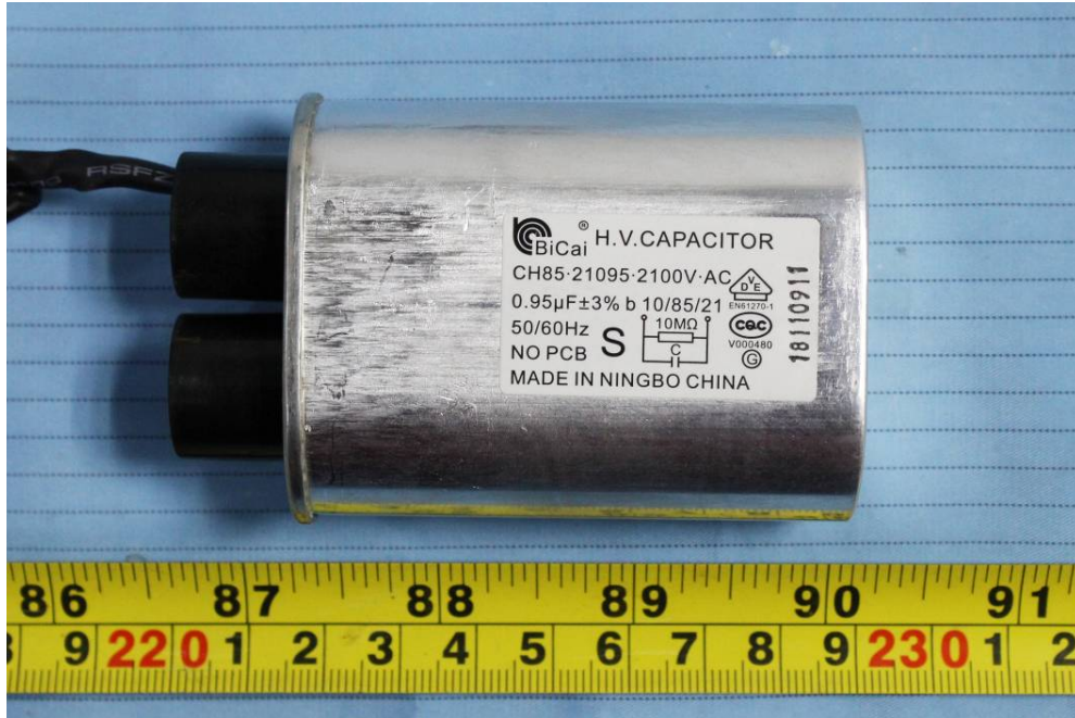
EUT – High Voltage Capacitor View
