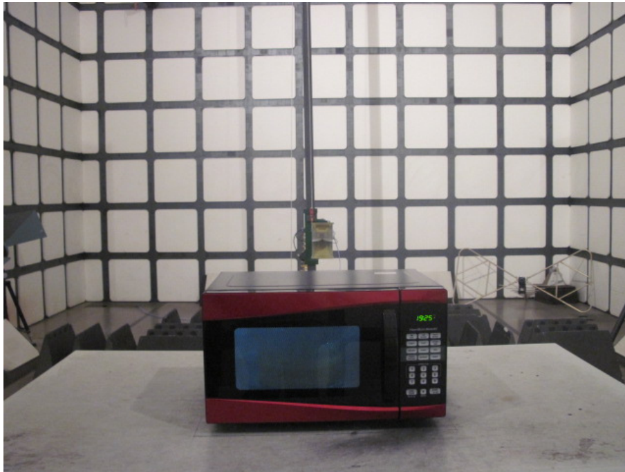
Operating Frequency Test Set-up
