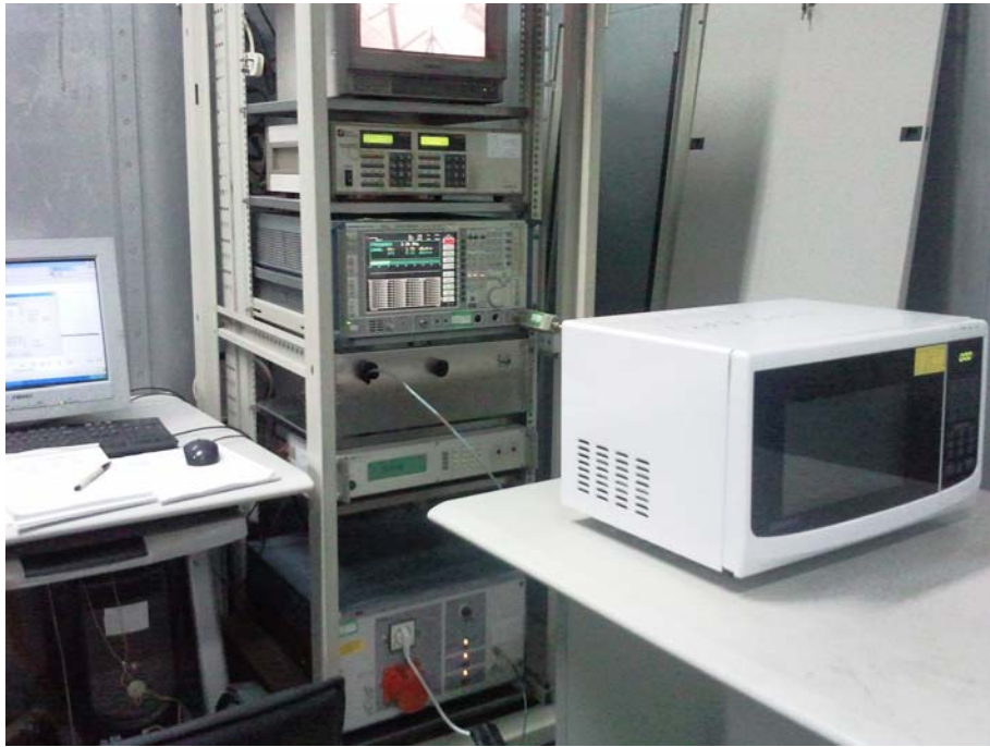
Conducted Emission Test Set-up
