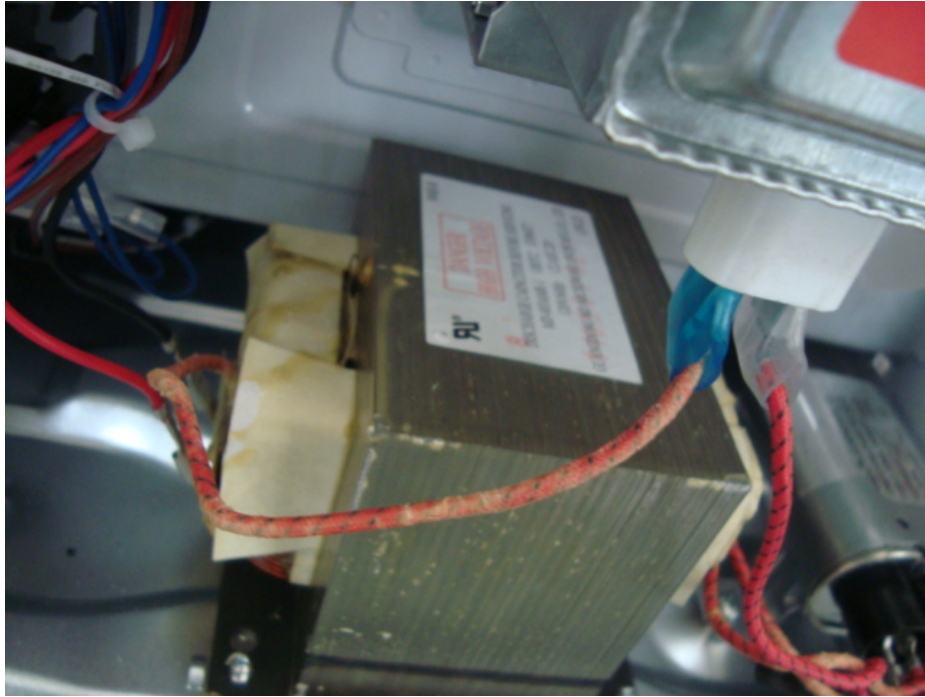
High-voltage Transformer View
