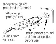
**CAUTION:** Attaching the adapter ground terminal to the wall receptacle cover screw does not ground the appliance unless the cover screw is metal, and not insulated, and the wall receptacle is grounded through the house wiring.
