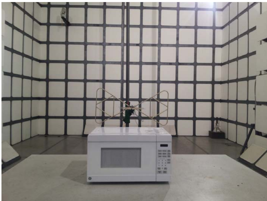
Radiated Emission Test Set-up (30 -1,000MHz)
