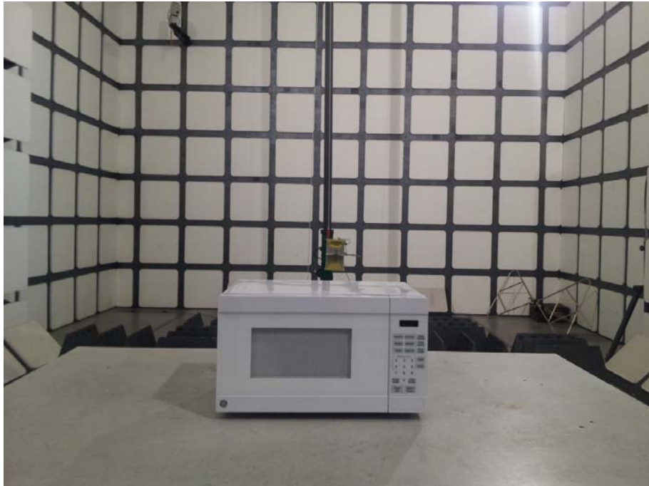
Operating Frequency Test Set-up
