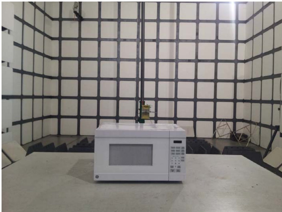
Radiated Emission Test Set-up (1-25GHz)
