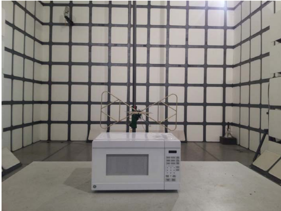
Radiated Emission Test Set-up (30 - 1,000MHz)
