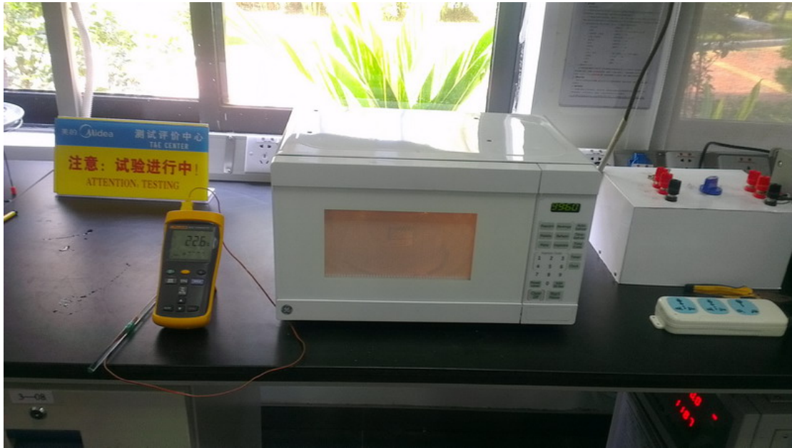
RF Output Power Test Set-Up
