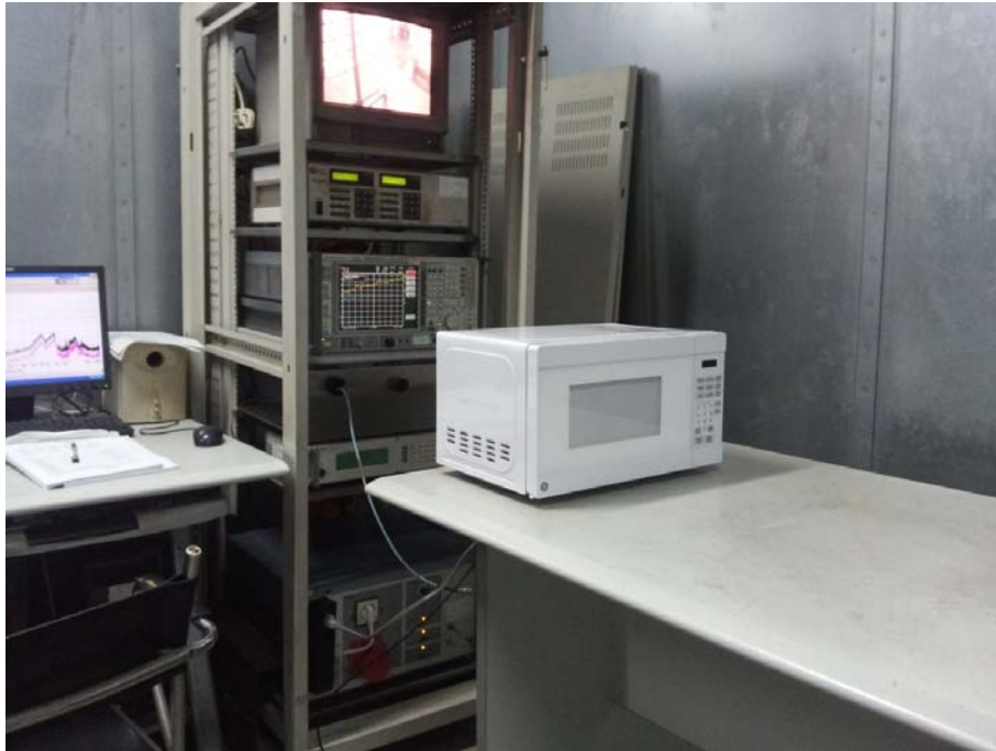
Conducted Emission Test Set-up
