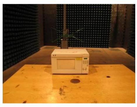
Set-up for radiation measurement above 1GHz
