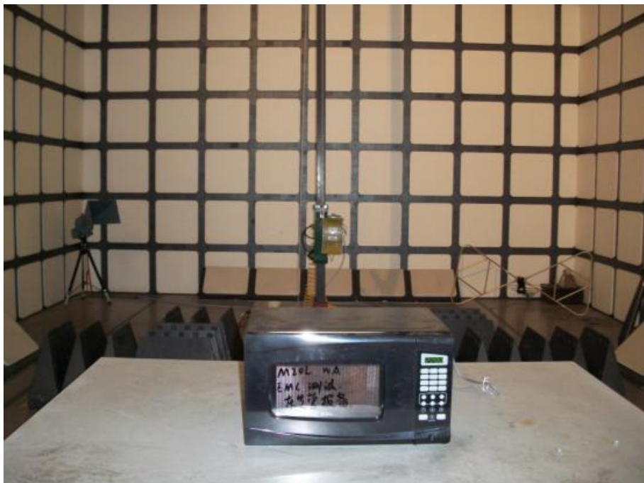
Radiated Emission Test Set-up (1-18GHz)
