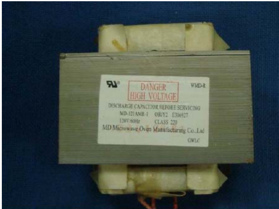
High-voltage Transformer View
