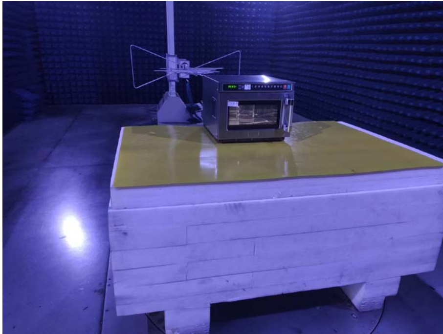
Photo of Radiated Emission Measurement Above 1GHz
