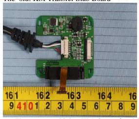
The new: combining KM60 transfer slab board into filter board
