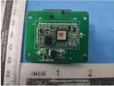
3. Adding alternative power supply board that combining KM60 transfer slab board into filter board The old: KM Transfer Slab Board
