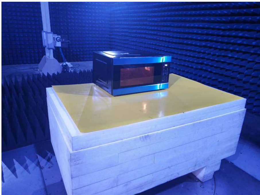
Photo of Radiated Emission Measurement Above 1GHz
