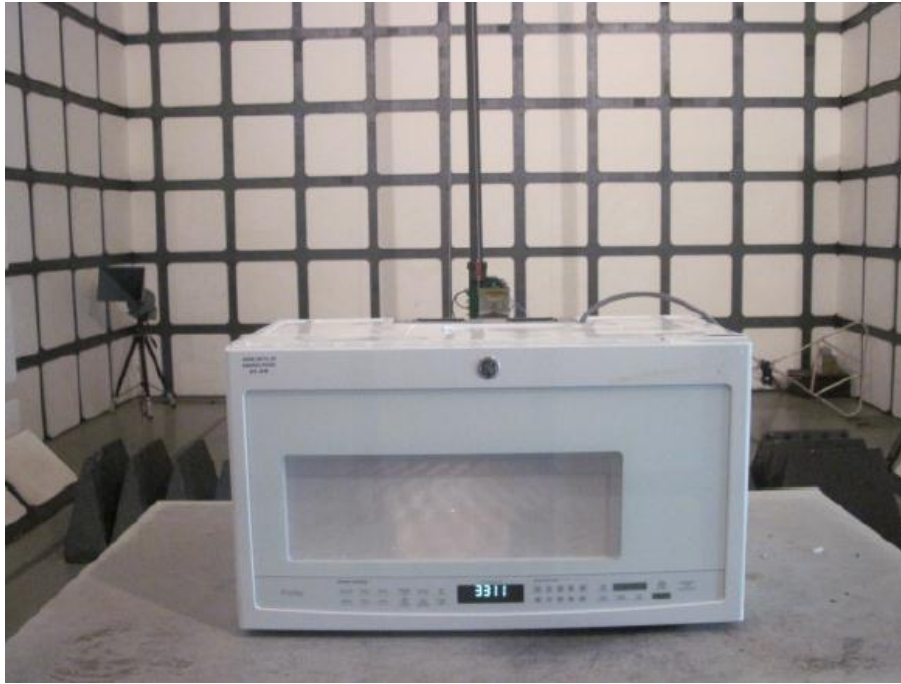
Radiated Emission Test Set-up (1-25GHz):
