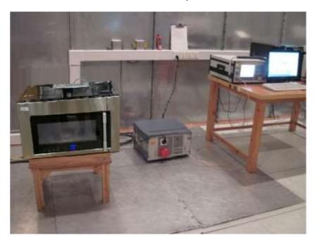
Radiated Emission Test Set-up (30 -1,000MHz):
