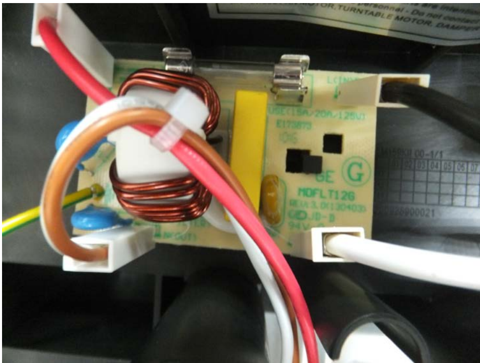
Power Filter Board Top View
