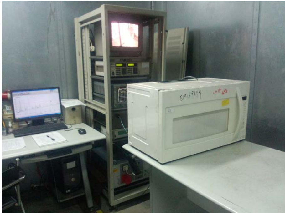
Conducted Emission Test Set-up
