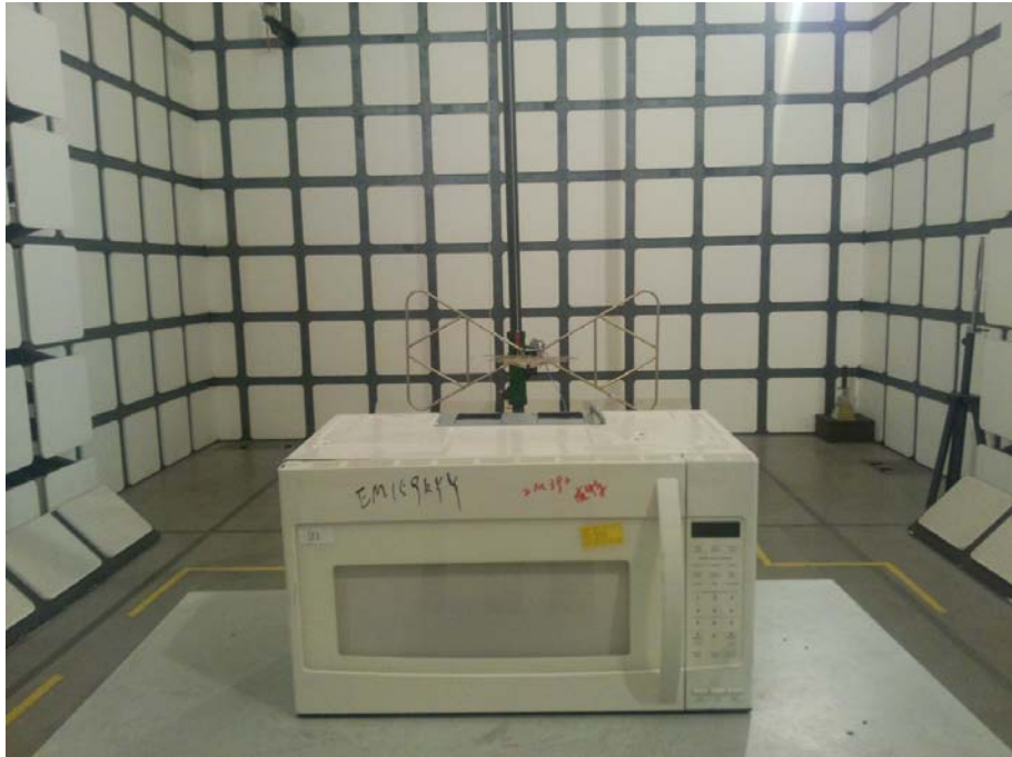
Radiated Emission Test Set-up (30 -1,000MHz)
