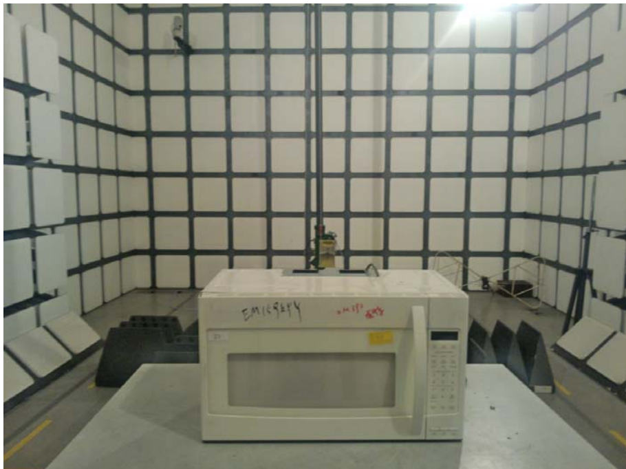
Radiated Emission Test Set-up (1-25GHz)
