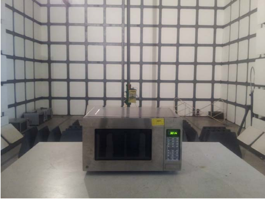
Operating Frequency Test Set-up
