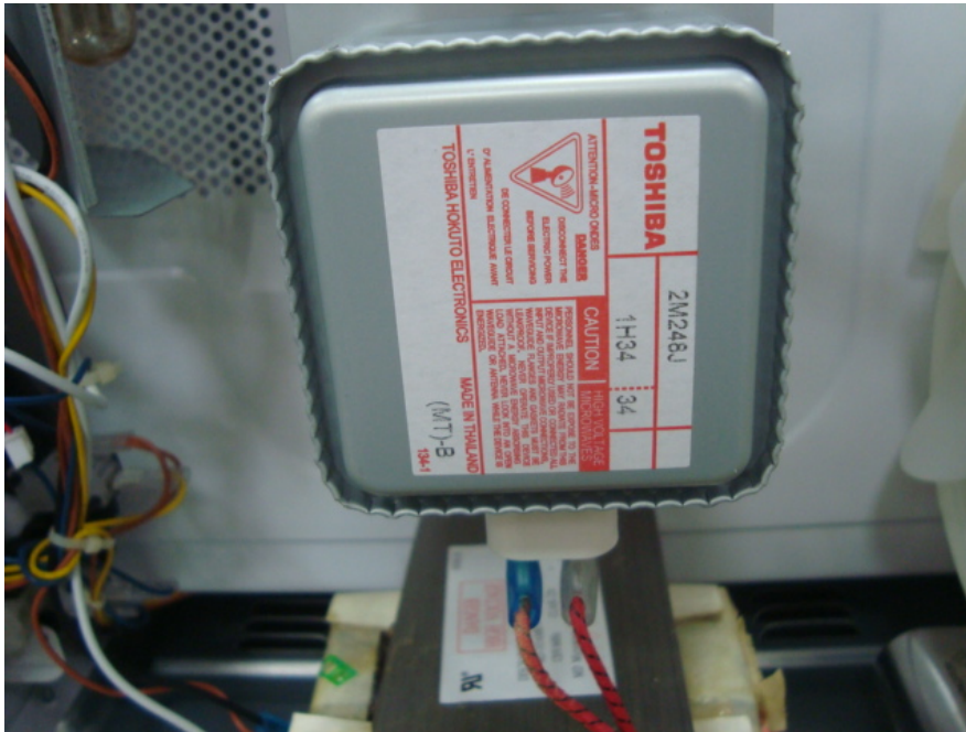
Magnetron Front View
