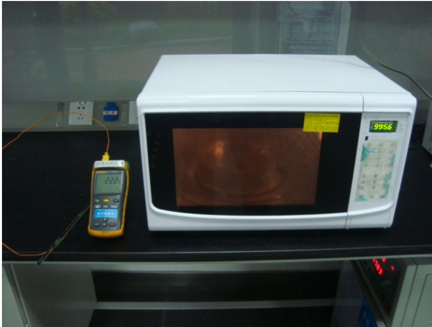
RF Output Power Test Set-Up
