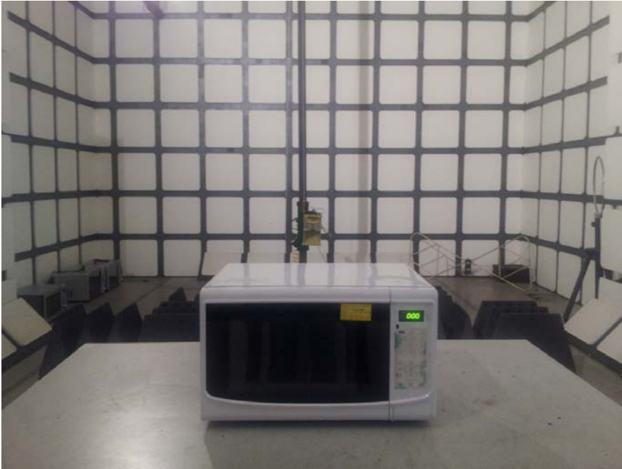
Operating Frequency Test Set-up
