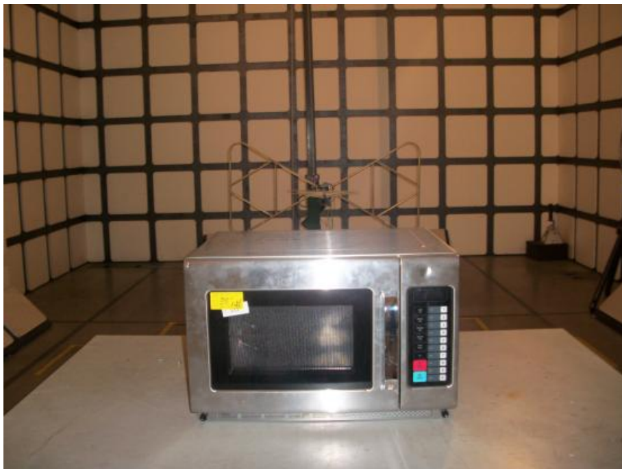
Radiated Emission Test Set-up (30 –1,000MHz)
