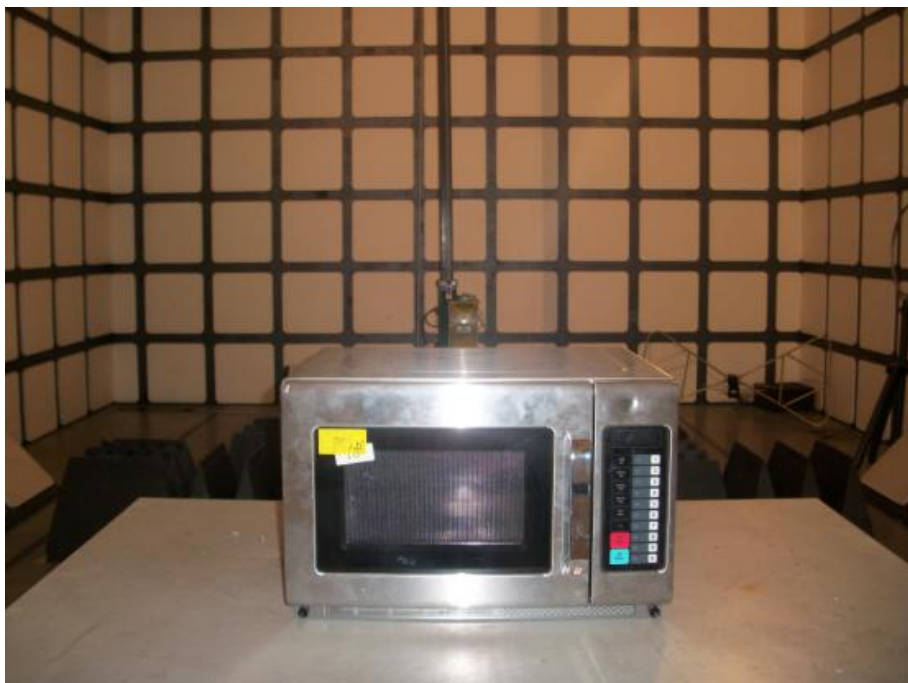
Radiated Emission Test Set-up (1–18GHz)
