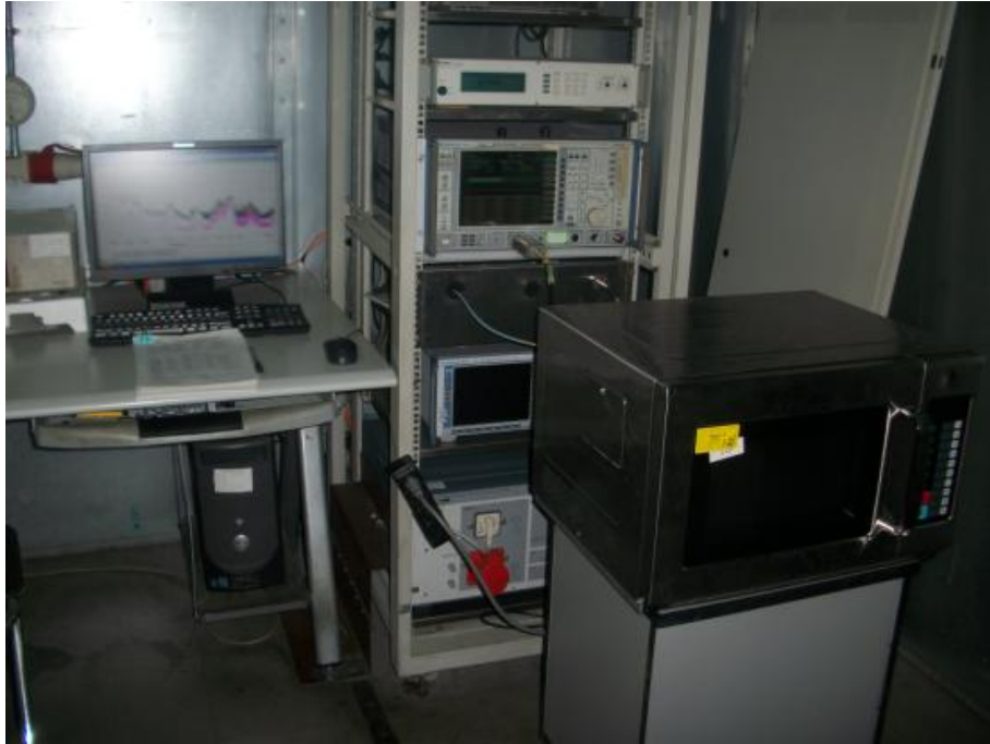
Conducted Emission Test Set-up
