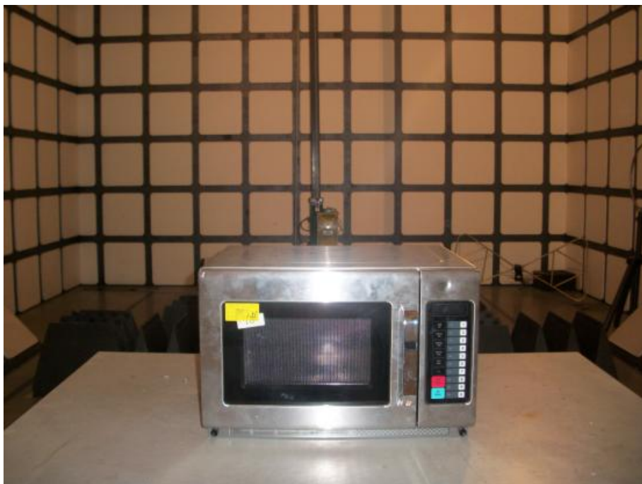
Operating Frequency Test Set-up
