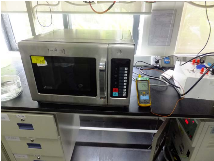
RF Output Power Test Set-Up
