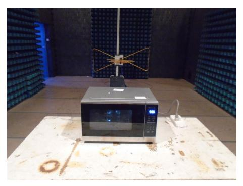
2. Radiated Emission Measurement above 1GHz
