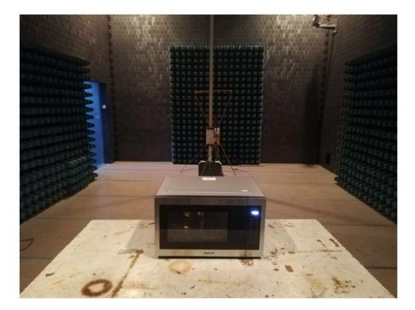
Radiated Emission Test Set-up (1-25GHz):
