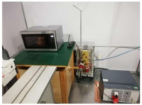
Radiated Emission Test Set-up (30 -1,000MHz):
