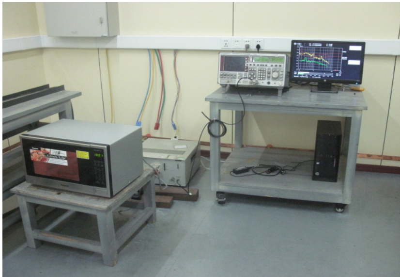
Conducted Emission Test Set-up
