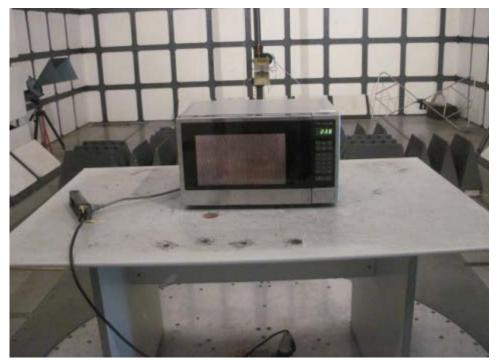
Radiated Emission Test Set-up (1-25GHz):
