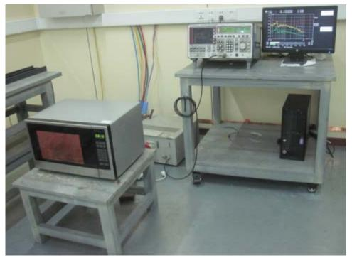
Radiated Emission Test Set-up (30-1000MHz):
