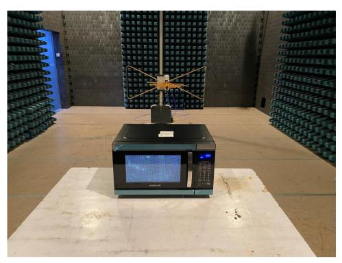
2. Radiated Emission Measurement above 1GHz
