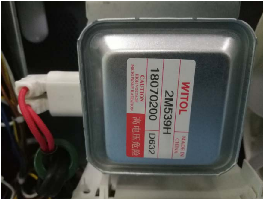
EUT – Magnetron View
