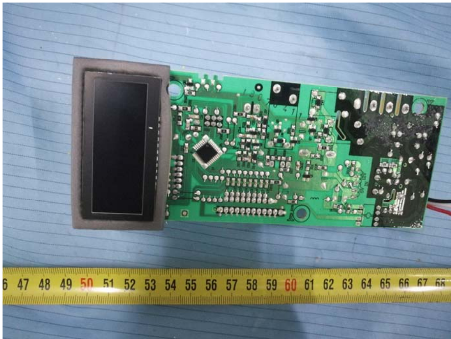
EUT – Main Board Bottom View
