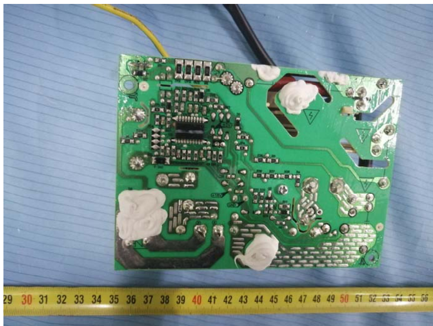
EUT – Transformer Bottom View
