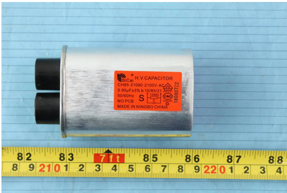
EUT –High Voltage Capacitor View
