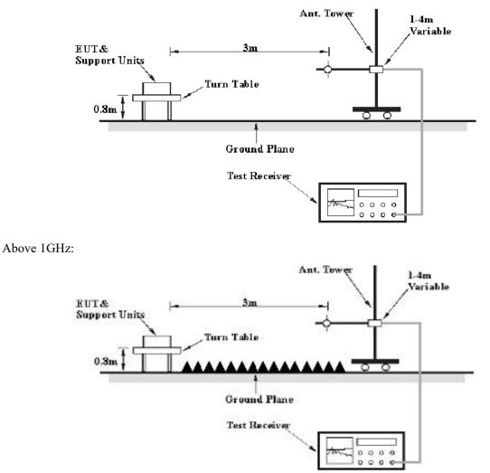
The radiated emission were performed in the 3 meters chamber test site, using the setup accordance with the FCC MP-5. The specification used was the FCC part 18 limits.
