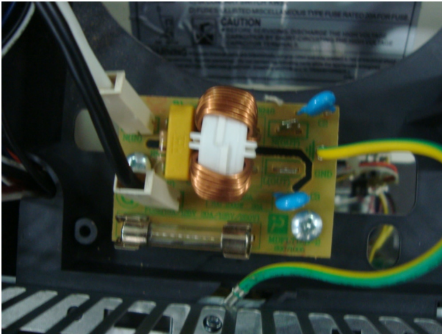
Power Filter Board Top View
