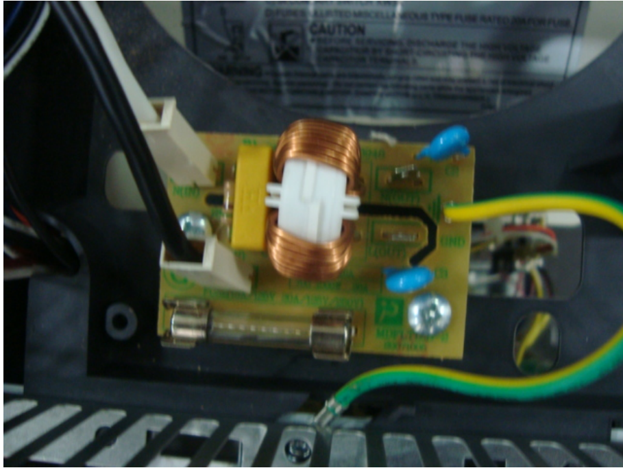
Power Filter Board -Front View
