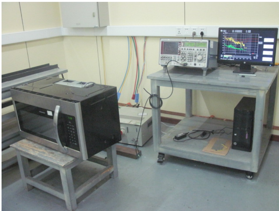
Conducted Emission Test Set-up
