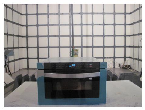
Radiated Emission Test Set-up (1-25GHz):
