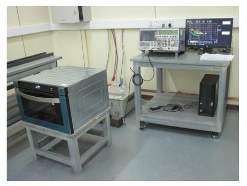
Radiated Emission Test Set-up (30 -1,000MHz):
